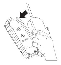
The CHARGE LED will blink to indicate that the Digital Security Code is set.
